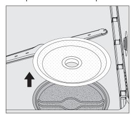
■ Remove the coarse filter and rinse under running water.
