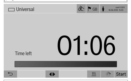
After selecting a programme, the time left for the chosen reprocessing programme is displayed. If the Display time left parameter is not activated in the web interface, the display switches to the already elapsed Duration of the reprocessing programme after programme start.
