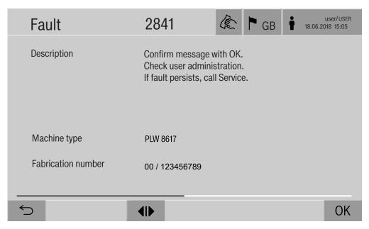
After a warning or fault button has been pressed in the message list, the message with information on rectifying the fault is indicated on the display.
