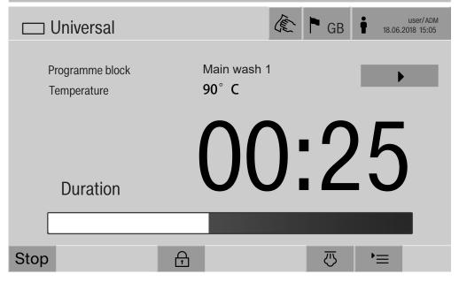
After the reprocessing programme has started, an additional ▶ button is displayed next to the programme block. The ▶ button has two functions:
