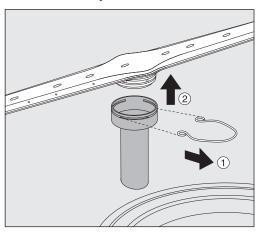
■ Loosen the securing clip on the spray arm connection and then pull the lower spray arm upwards and the upper spray arm downwards.
